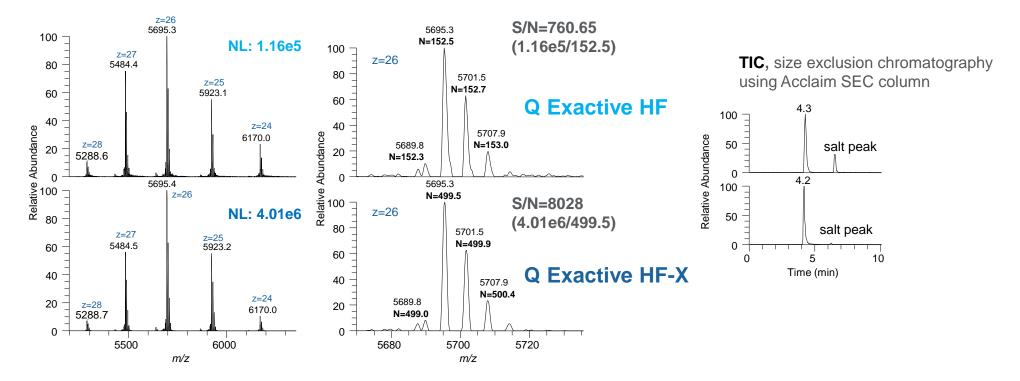
SEC-LC/MS analysis of intact Trastuzumab monoclonal antibody using Acclaim SEC column, 4.6 x 300 mm, 300  $\mu$ l/min flow rate, 50 mM ammonium acetate. Full MS, HMR mode, m/z 2500–8000, resolution setting 30k, 10  $\mu$ scans. Spectra show an average of 3 scans (10  $\mu$ scans each).
