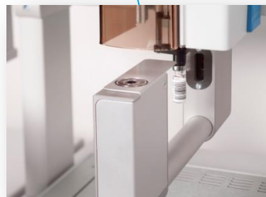
Barcode reader for sample tracking
