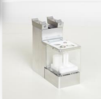
Vortexer for Intensive sample mix
