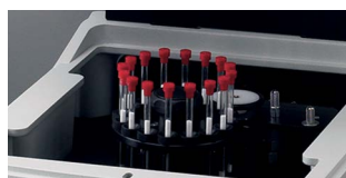
The Carousel Autosampler Sampling accessory for the DXR3 SmartRaman Spectrometer
